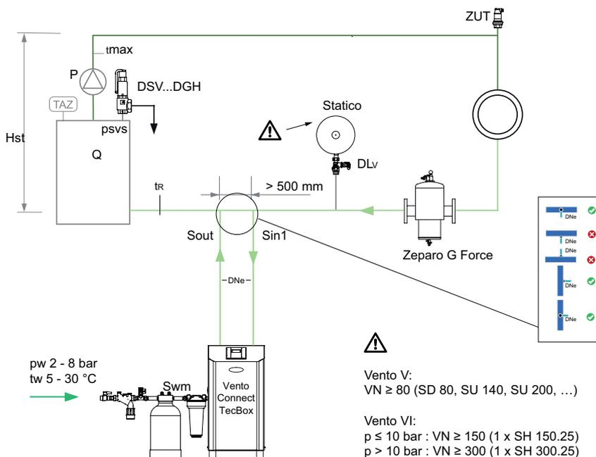
**Zeparo G-Force** for the central separation of sludge.
