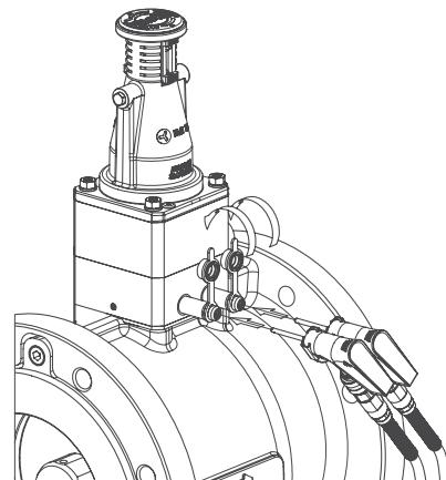
Connect IMI TA balancing instrument to the measuring points and measure  $\Delta p_L$ .
