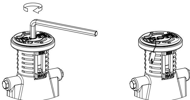
1. Use a 5 mm allen key for setting. Turn clockwise to increase the setting, see table "Setting table" and "kPa/turn". Each rib on the pilot correspond to the different settings in the "Setting table".
