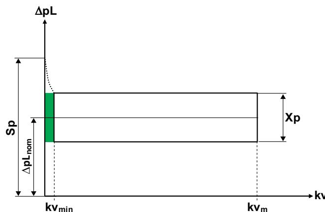
$Sp$  = Sealing pressure, the increase of  $\Delta pL$  in kPa when a  $\Delta p$  controller controls  $\Delta pL$  from  $Kv_{min}$  down to zero flow.
