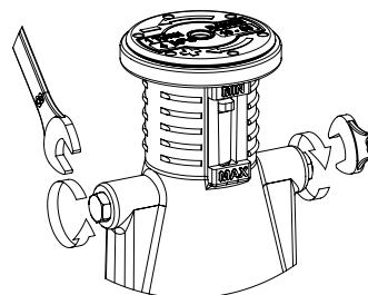
To vent the valve, open the topmost venting screw.
