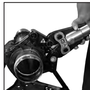
Figure 8: Placement of adapter jaw into pressing chain
