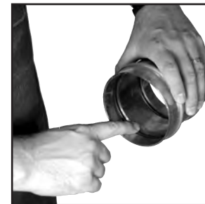
Figure 5: Check for EPDM seal
