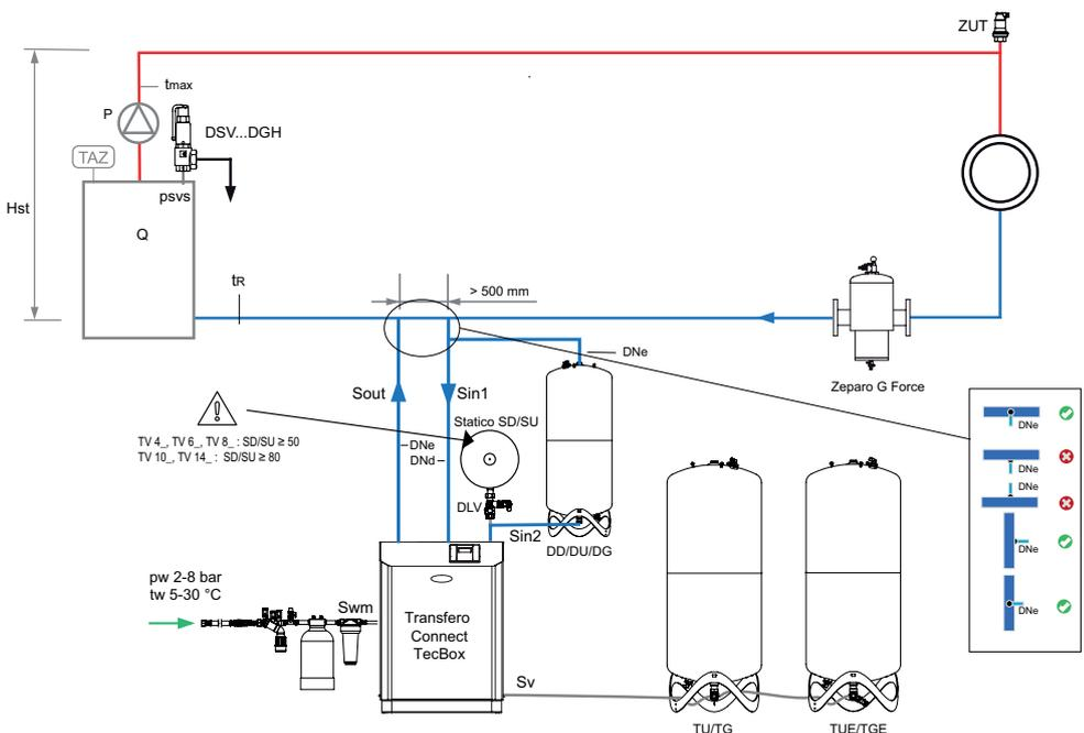
**Zeparo G-Force** for the central separation of sludge.
