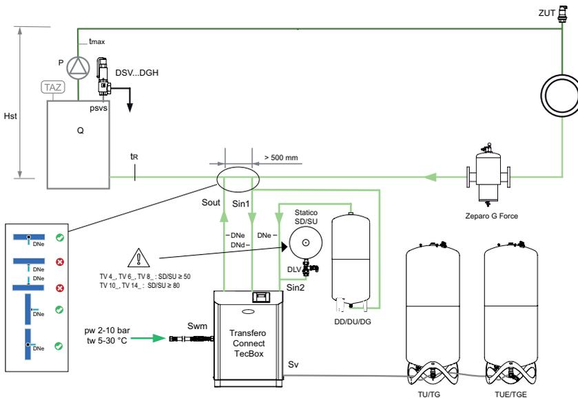
**Zeparo G-Force** for the central separation of sludge.
