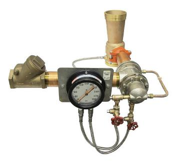
The In-Line Balanced Pressure (ILBP) Proportioner is a foam proportioning device which is used to balance the higher foam concentrate pressure to the lower system water pressure on pilot pressure regulating systems or foam pump proportioning systems. The ILBP is particularly useful in providing accurate proportioning at multiple riser locations that are situated remotely from the central foam concentrate storage tank.
