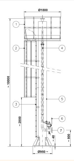
Other heights available on request - dimensions for 10 m tower -Fabricated according to EN14122
